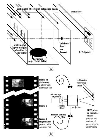
Fig. 4. Making the recording of the way the author's dwelling responds to light: (a) With a scale model. (b) With a sequence of 41 pictures taken at different times of day, using the sun shining in the windows as the sole source of illumination; the sequence of images was later multiplexed onto a holographic plate with a 35-mm motion picture projector illuminated with laser light.
