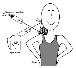
Fig. 1. Hypothetical measurement of the response of a scene to light, using a spot meter and an idealized spotlight (producing a single ray). The entire measurement space provides all information necessary to reconstruct the scene from any viewpoint under any illumination.
